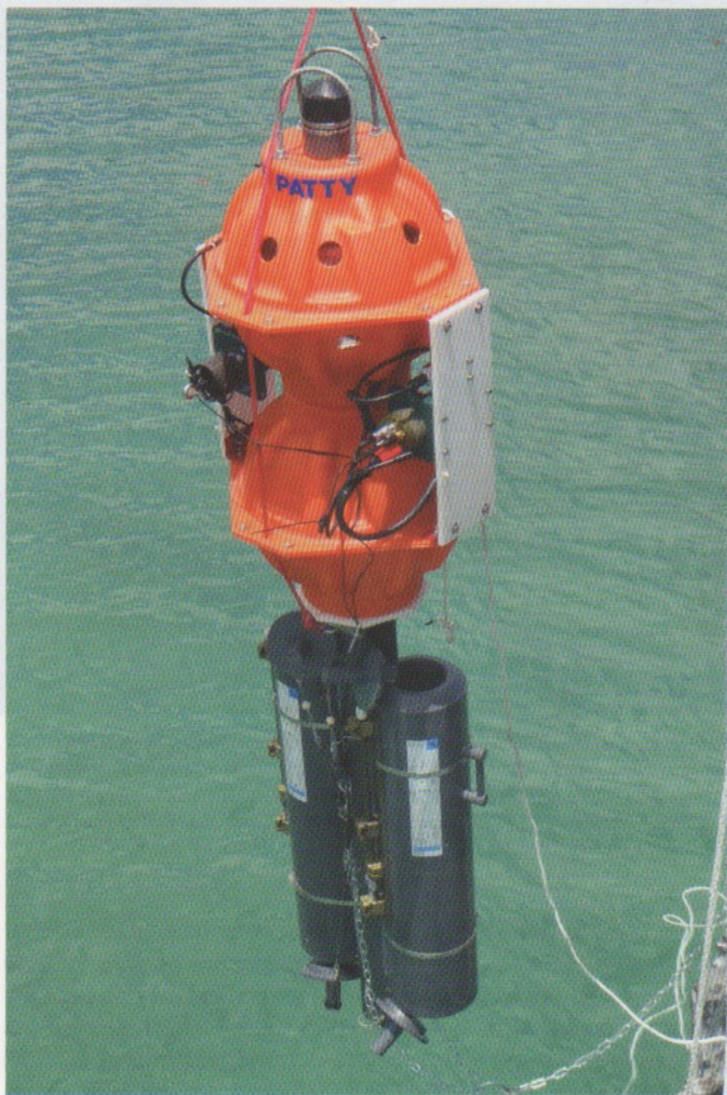
DOV Patty, suspended over Agana Harbor, Guam, prior to deployment in the Sirena Deep of the Mariana Trench in 2011. In this scalable design, the upper sphere contains the acoustic command/control system plus surface recovery beacons. A second sphere is added to offset the weight of the lower payload pod. Side panels provide mounting surfaces for sensors and an external back-up timer.
