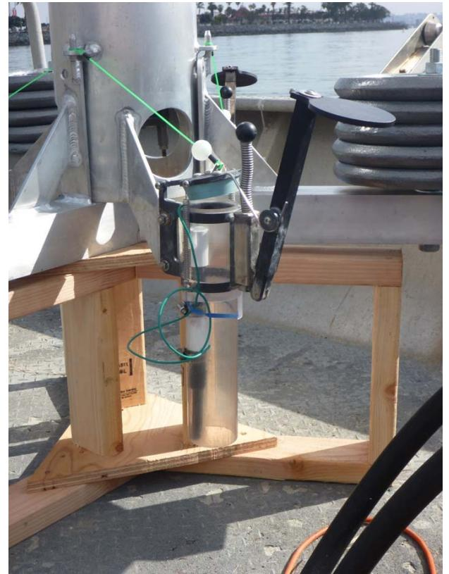
Fig. 2. Sediment retaining tube with open covers and MFC anode. Ascent of cylinder away from ballast platform releases covers to close via springs.
