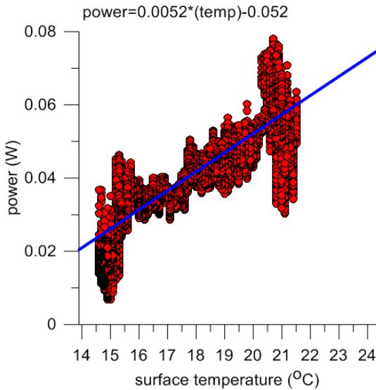
Fig 10. Effect of temperature on MFC output from MCRD sediments in situ.
