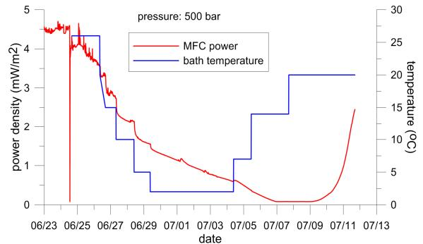
Fig 9. Effect of temperature on MFC output from MCRD sediment at 500 bar.
