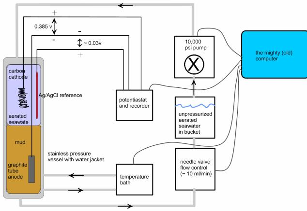
Fig. 4. Laboratory MFC in pressure vessel, meant to mimic deep sea conditions of in situ measurements.
