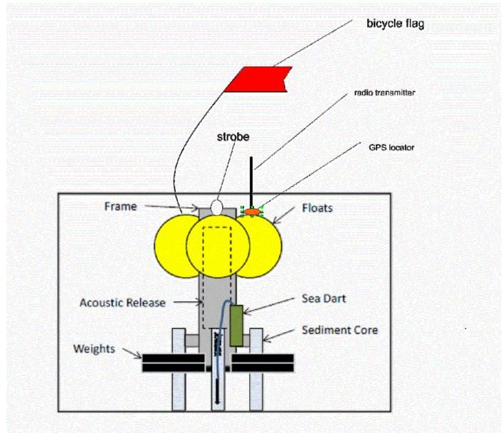
Fig. 1. Schematic of free vehicle that buries MFC anodes in sediment, records MFC power, collects sediment samples, and returns to the surface after dumping ballast via an acoustic release.
