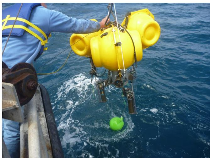
Fig. 3. Recovery of Microbial Fuel Cell vehicle with full sediment tubes.
