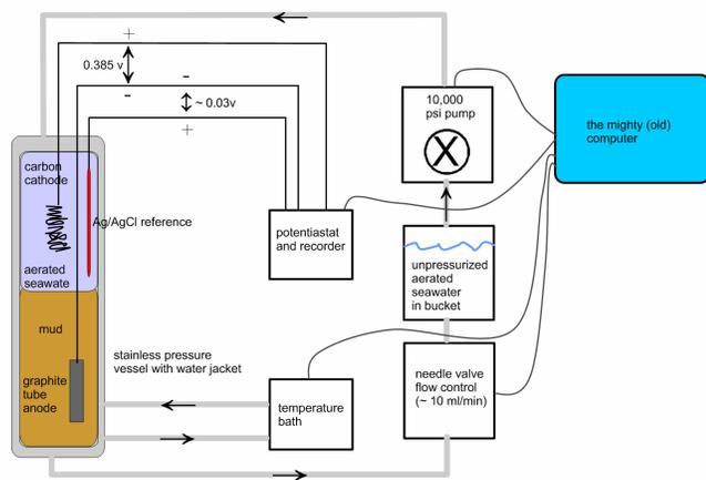
Fig. 4. Laboratory MFC in pressure vessel, meant to mimic deep sea conditions of in situ measurements.
