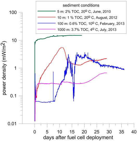
Fig 6. MFC output at various depths and temperatures.
