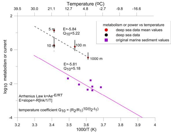
Fig 7. Arrhenius plot of metabolic activity and MFC output versus temperature. Upper regression line and data from Fig 6.
