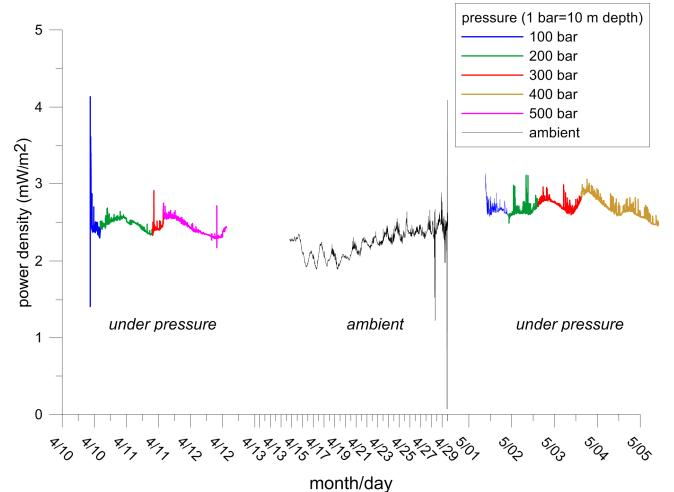
Fig 8. Effects of various pressure regimes on MFC output from MCRD sediment at ambient (~20 °C) temperature.
