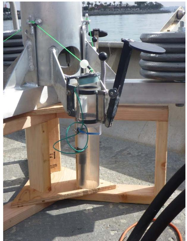
Fig. 2. Sediment retaining tube with open covers and MFC anode. Ascent of cylinder from ballast platform releases covers to close via springs.
