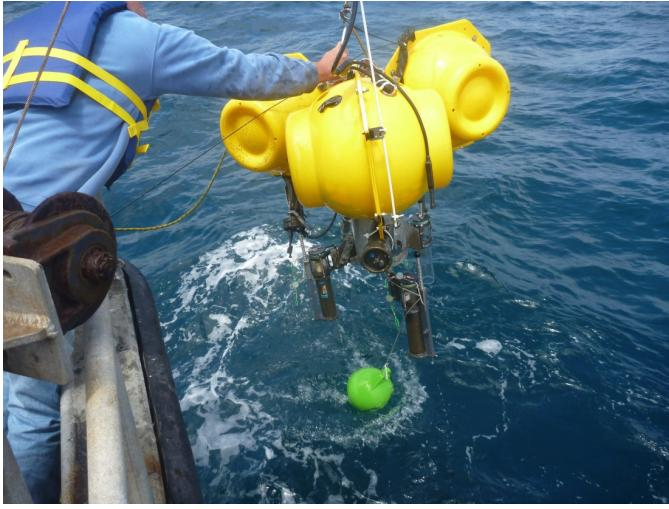
Fig. 3. Recovery of Microbial Fuel Cell vehicle with full sediment tubes.
