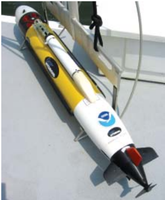
Fig. 1. The Office of Coast Survey's REMUS AUV
