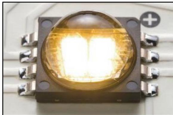
Figure 2. The Cree MCE 4-chip LED allows for more light from a single package while each die operates at a cooler temperature. [10]
