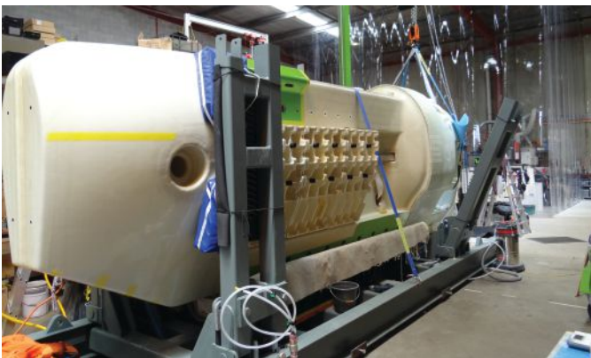
Figure 3. The DSC main spar before painting made of ISOFloat syntactic. Photo by Tim Bulman, used with permission, Earthship LLC.
