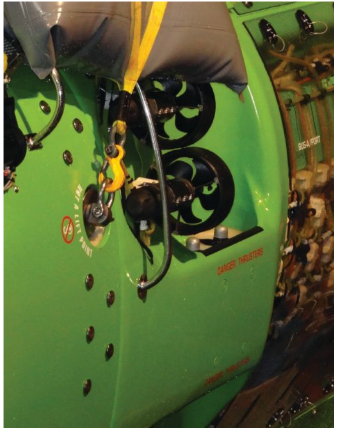
Figure 7. The DSC on deck with vertical thrusters and LiPo battery pods visible. Photo by Tim Bulman, used with permission, Earthship LLC.
