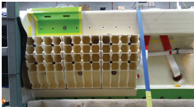
Figure 4. The PBOF LiPO slots made of ISOFloat syntactic. Photo by Ben Grant, used with permission, Earthship LLC.
