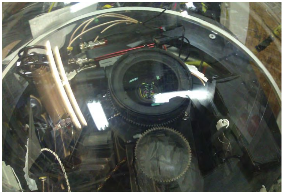
Figure 2. A Canon 5D camera is seen through the optically polished Nautilus Marine Vitrovex glass housing. Photo by Charlie Arneson, used with permission, Earthship Productions.
