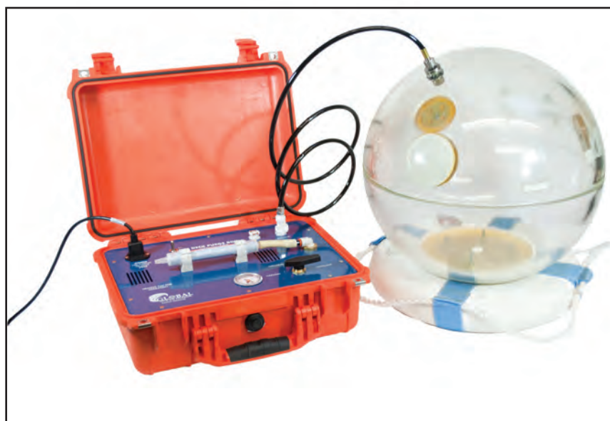
Figure 2. This Deck Purge Box is an example of a safe and field-tested way to dynamically eliminate excess moisture in undersea instrument housings.
