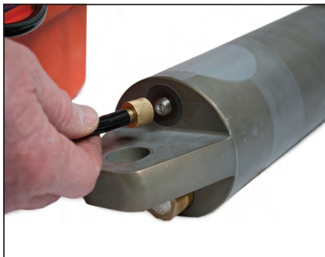
Figure 4. A self-sealing purge port installed in an aluminum pressure case with the pressure proof cap removed. The center core check valve is seen.
