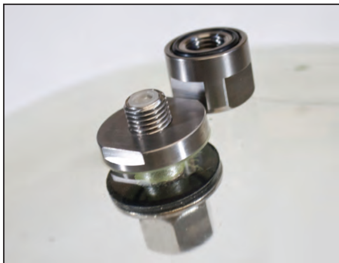
Figure 3. A self-sealing purge port installed in a glass sphere with the pressure proof cap removed. The center core check valve is seen. With the core check valve sealed, the operator has time to carefully clean and install the face seal o-ring seen on the pressure proof cap in the background.
