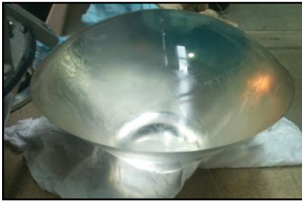
Figure 6. The DSC’s conic acrylic viewport. Photo by Bruce Sutphen. Used with Permission, Earthship LLC.
