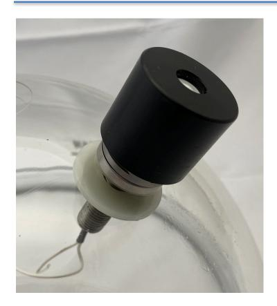
Turn instruments on or off after deployment using the Global Ocean Design **Pressure Activated Switch for spheres**. The switch is selected to be either "ON" or "OFF" at the surface. As the switch is carried below 2-5 atmospheres deep, it switches to the alternate position. On return to the surface, the switch toggles back to the initial position.
