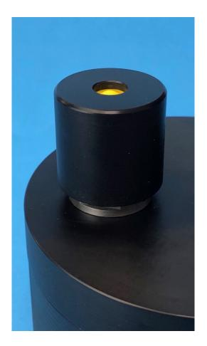
Turn instruments on or off after deployment using the Global Ocean Design **Pressure Activated Switch for end caps**. The switch is selected to be either "ON" or "OFF" at the surface. As the switch is carried below 2-5 atmospheres deep, it switches to the alternate position. On return to the surface, the switch toggles back to the initial position.
