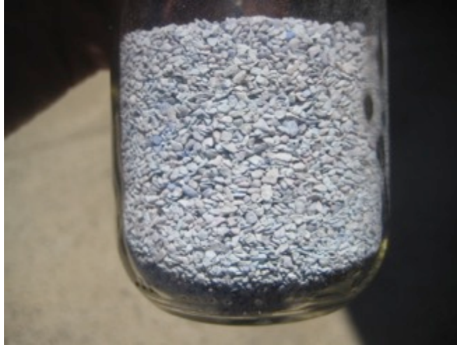
Figure 12. Indicating desiccant in natural daylight.
