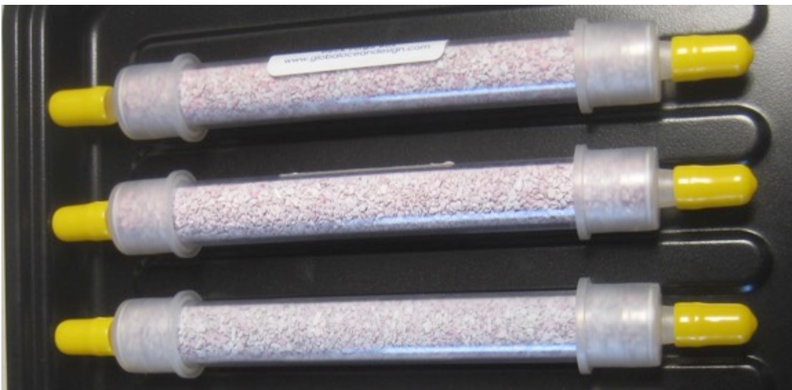
Figure 1. Spent cartridges. These have adsorbed as much moisture as they can, turning the indicating desiccant from blue to pink.
