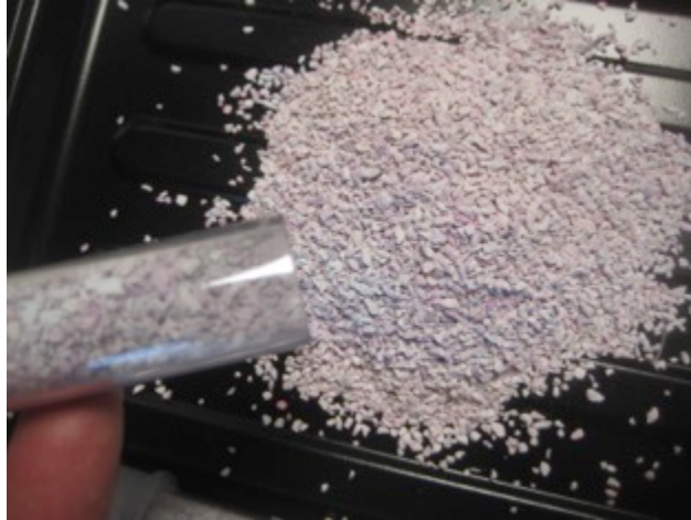
Figure 4. Empty the granules onto a glass or metal cookie sheet. Spread to a thin layer.
